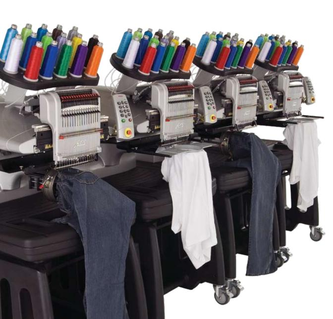
Individual AMAYA XTS units are connected by ethernet cable, not by a conventional rigid framework.
